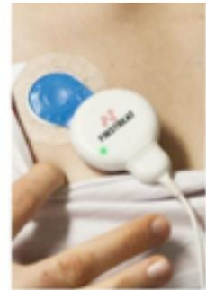
d. The measurement starts automatically when the device is attached.
